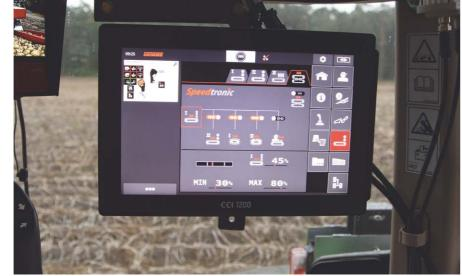
MemoryControl allows the central adjustment of the drives and separators. It is possible to save settings such as speed, adjustable angles and percentage values for different harvesting conditions and recall these quickly if required. Up to 8 programs can be saved and allow you to set your harvesting performance from gentle to output-oriented.
