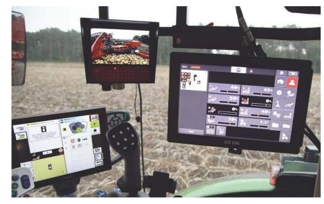
The optional Speedtronic automatically adjusts the speed of the separators and the picking table to the harvesting conditions, thus increasing crop protection while at the same time increasing area output and relieving the strain on the driver.
