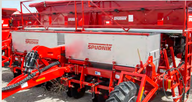
Dry Fertilizer The fertilizer is applied in two bands, next to the seed piece.
