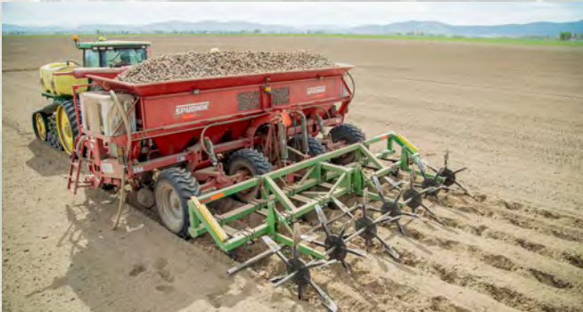
Single Pass Operation Fertilizing, planting, hilling, applying chemicals and dammer dyking in one pass.
