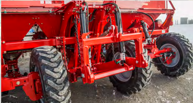
Three Point Hitch Mount any cultivator or hiller to your planter.
