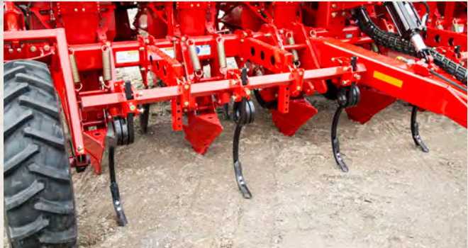
Front Tool Bar Softens the soil to keep the planting depth more consistent.
